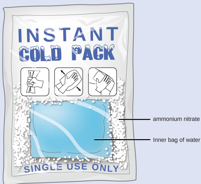
Figure 5.16 An instant cold pack consists of a bag containing solid ammonium nitrate and a second bag of water. When the bag of water is broken, the pack becomes cold because the dissolution of ammonium nitrate is an endothermic process that removes thermal energy from the water. The cold pack then removes thermal energy from your body.
